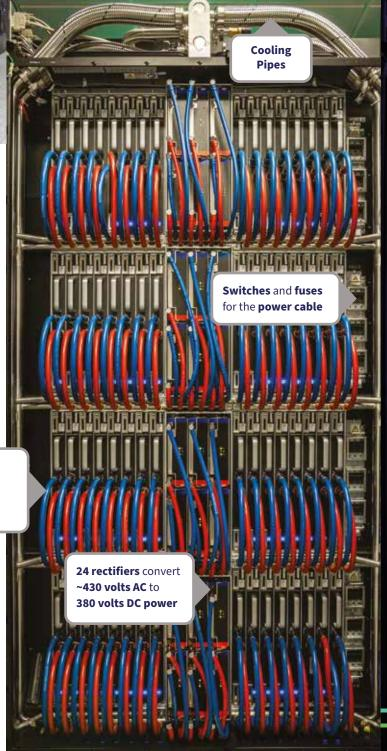
Each blade has **4 nodes**Each node has **two 64-core CPUs**A total of **32,768 cores per cabinet**
